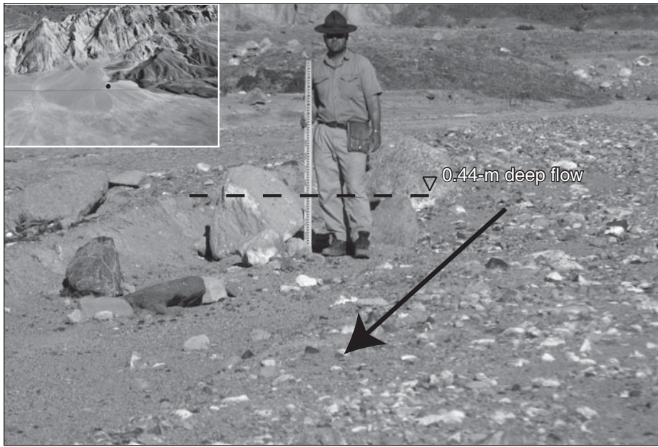
Figure 23. View up road inundated by Desolation Canyon fan channel in 2004, Death Valley, California. A 0.6-m boulder (next to author) rests atop an old road surface, which slopes at 0.043; a trim line on the road berm to the left of this boulder indicates a maximum flow depth of 0.44 m. The image indicates that exceptionally large particles may be mobile on steep, finer grained fan channels where flow approaches maximum particle diameter. Observed decreases in maximum particle size down traction-dominated fans may be statements about decreasing flow depth.
